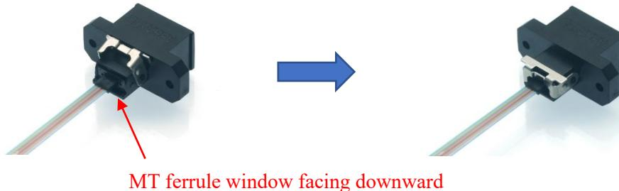
Step 1: Insert the MT ferrule ② into the MT port of the adapter body ①, and then rotate the swing clip to lock the MT ferrule ② in place.
