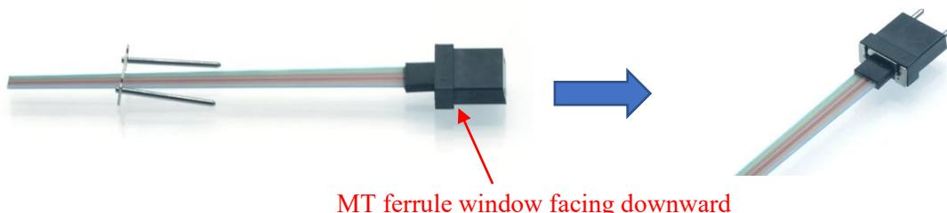
Step 2: Insert the MT ferrule/guide pin into the MT port of the adapter body ① and rotate the swing clip to lock the MT ferrule ② in place.
