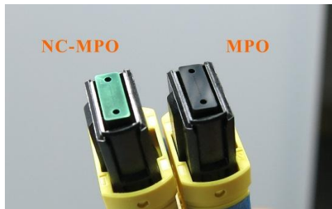
Figure 1. Non-contact MPO fiber connector (left) has an anti-reflective coating on the end face, compared to a conventional contact MPO connector (right)
