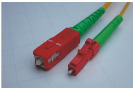
"Non-Contact" (NC) fiber connector is the next generation optical fiber connector invented by Arrayed Fiberoptics, where there is no contact between fiber surfaces. There are two key elements in the NC connector, 1) the fiber surface is recessed, 2) the fiber surface has an anti-reflection coating. It offers vastly improved optical performance and longevity.
